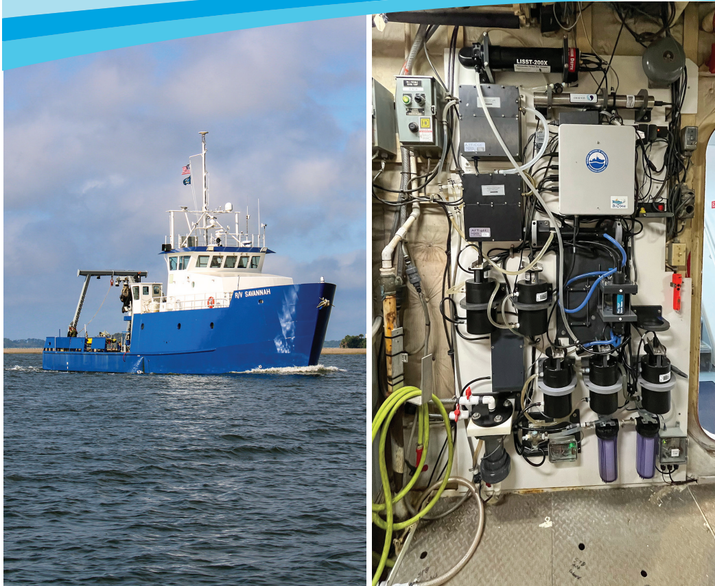
The new flow-through system aboard the R/V Savannah uses more than a dozen instruments to continuously measure biogeochemical parameters on the ocean's surface. (Photo by Jackson K. Schroeder)
